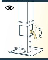
You can never be too careful. A **safety system** on the extension locking bolt provides the best guarantee against the foot dropping during
