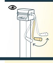
The handle is a protruding part. The quick lock/unlock **system**, available on request, prevents any movement of the handle due to impact or vibration.
