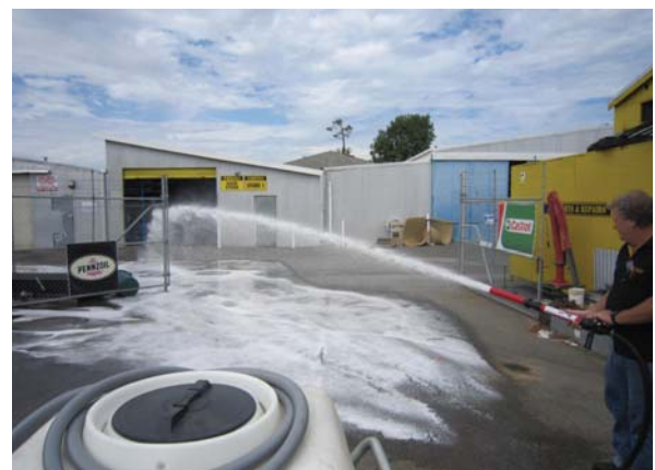
Foam-fast in Operation 1" nozzle
