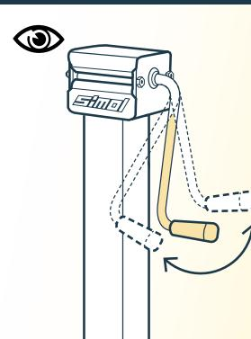
The handle is a protruding part. The quick lock/unlock system, available on request, prevents any movement of the handle due to impact or vibration.
