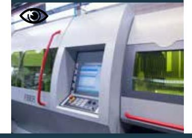
System developed for **high-speed cutting of tubes of different materials.**
