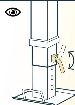
You can never be too careful. A safety system on the extension locking bolt provides the best guarantee against the foot dropping during manoeuvres.
